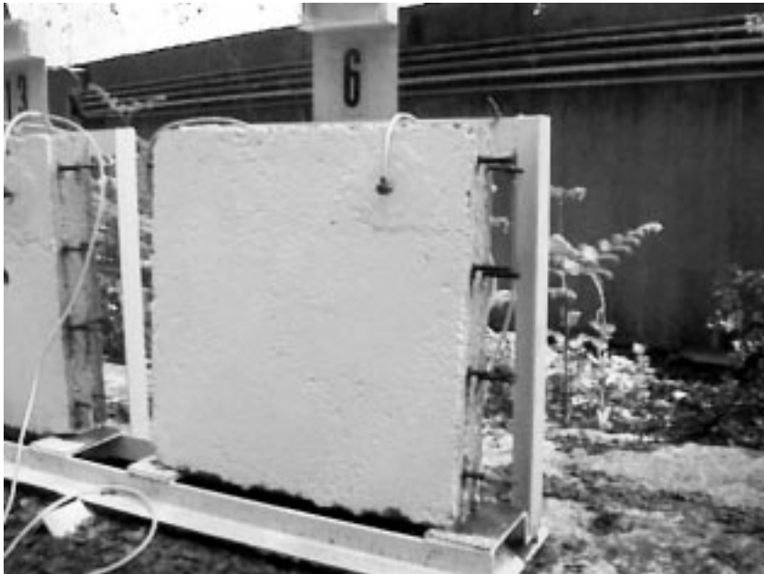
Figure 4: Sprayed zinc coated concrete specimen with organic topcoating
